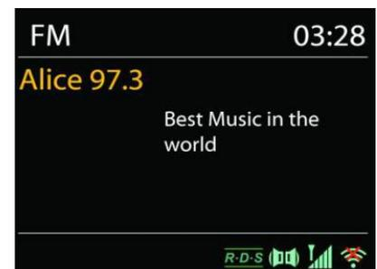
To full scan, press “**INTRO**” remote key. The frequency display starts to run and scans the FM full band and saves the found stations as presets.
