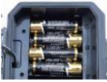
① Install Batteries
