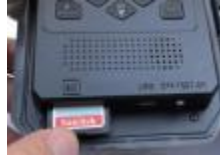
② Install micro SD Card
